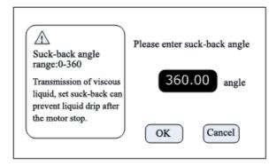
Click the **Setting** button in the main interface, then click **Suck-Back** button to enter the back suction angle setting interface. Click **angle** button, enter suck-back angle then click **ENT**. This can set all suck-back angle when motor stop running, except **dispensing** is **ON**.
